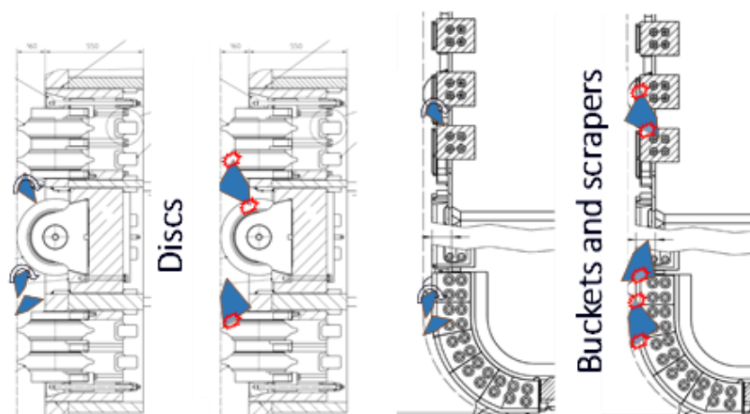
Figure 10. Representation of the effect of block sizes on damages to tools due to accumulation of material in front of the cutterhead.
