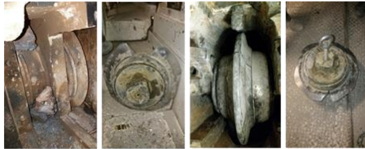
Figure 6. Damage on discs due to overloading and impact loads.
